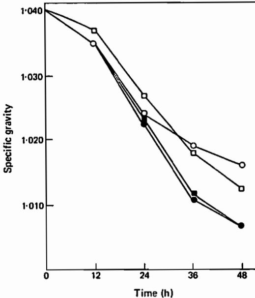
Fig. 2.—Change in specific gravity during fermentation of wort by oxygen-requiring *Saccharomyces cerevisiae* (NCYC 1236) in relation to the content of ergosterol: no ergosterol (○), 1 ppm (□), 10 ppm (●), 18, 70, 140 ppm (■).
