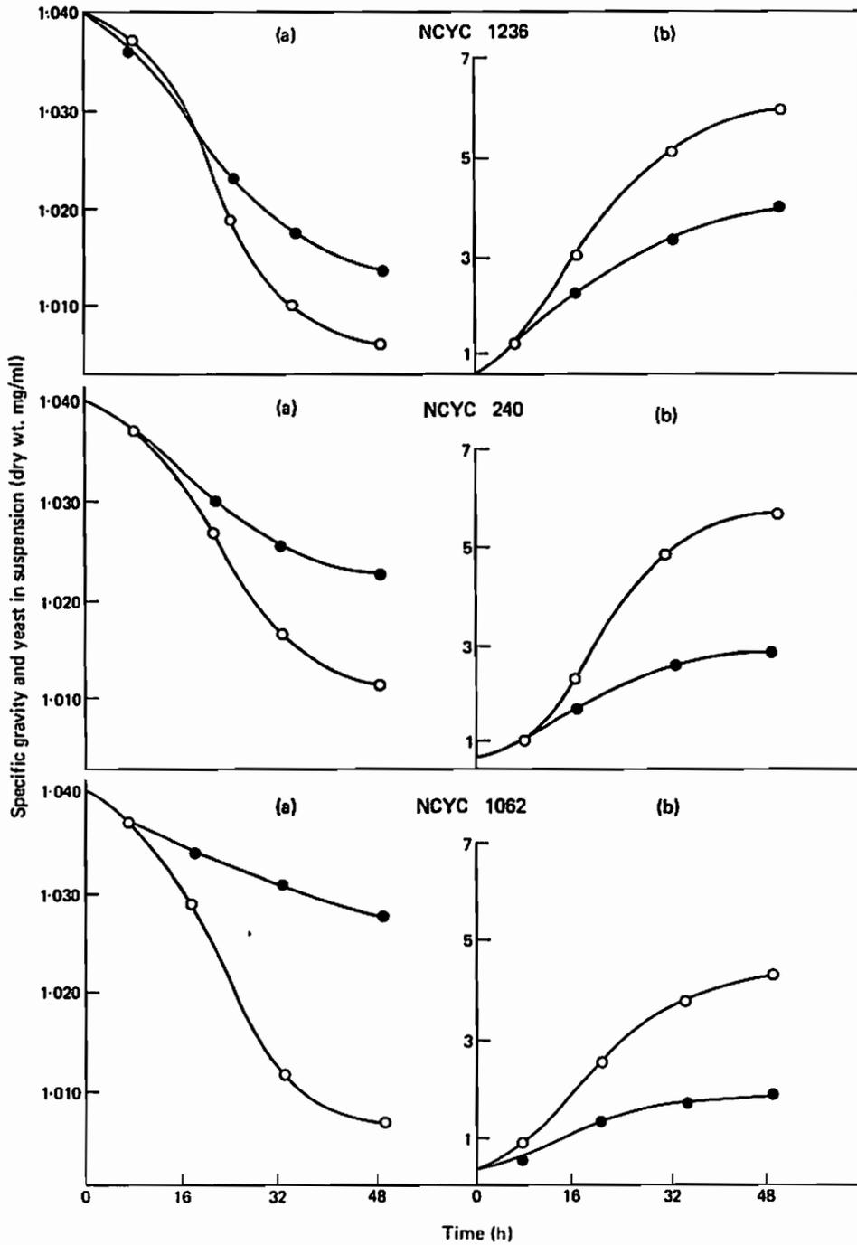
Fig. 1.—Changes during fermentation in (a) specific gravity and (b) yeast dry weight when de-aerated wort is pitched with cells with (●) and without (○) requirement for oxygen. The results for the other yeast strains examined follow the pattern shown for strain 240.
