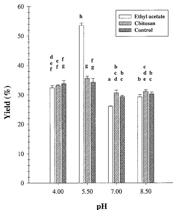
Fig. 2. Effect of chemical agents and pH on yeast extracts yields following 24 h of incubation at  $48^\circ\text{C}$ . Letters were added at the top of columns to indicate statistical differences. Columns that have the same letter are not significantly different ( $P > 0.05$ ).
