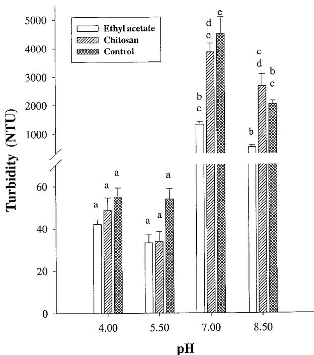
Fig. 6. Effect of chemical agents and pH on the turbidity of yeast extracts obtained after 24 h of incubation at 48°C. Letters were added at the top of columns to indicate statistical differences. Columns that have the same letter are not significantly different ( $P > 0.05$ ).
