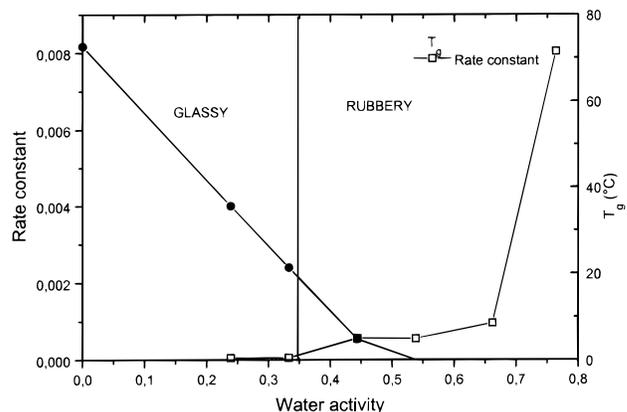
**Figure 3.** Relationships between water activity, glass transition temperature  $T_g$ , and reaction rates.
